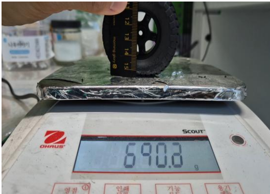
Fig. 37. Measuring Tire's Stiffness Value
