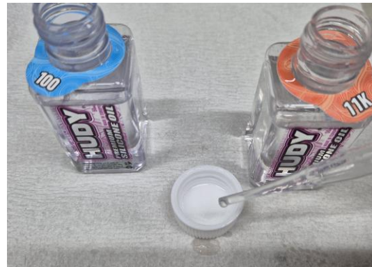
Fig. 42. Mixing Two Suspension Oils
