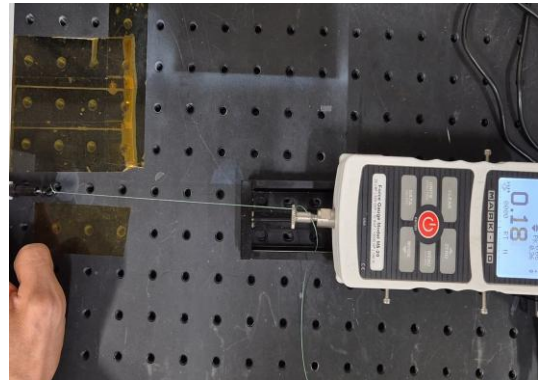
Fig. 38. Measuring Damping Coefficient
